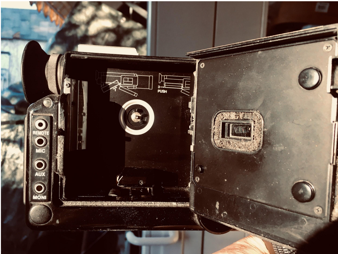
Above, the Canon 814XL-S Super 8 camera produced in Japan from 1978 to 1983. Below is the camera opened and it is possible to see where the cartridge is inserted. Photography taken at Kahl Film and TV e.K. Studio in Brühl, Germany, on February 15, 2019.
